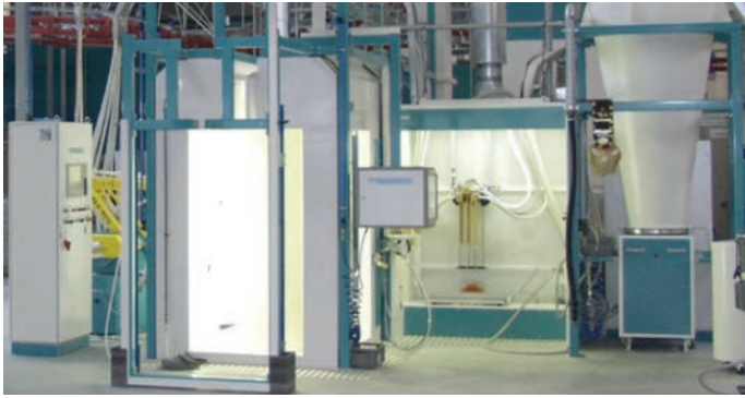
FCC Fast Colour Change System - Improves productivity through decreasing colour change time from 12 to 6 mins during recovery operation.
