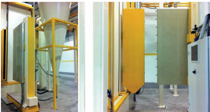
FCB Belt Powder System - Fast colour change system for clean room applications. Cleaning by suction system.
