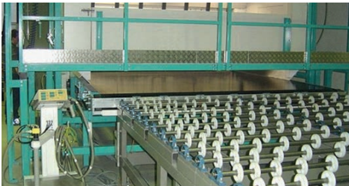
FCH Horizontal Powder System - Horizontal system for glass or flat coating.
